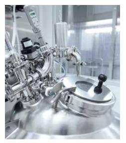
Temperature sensor with fermenter connector
