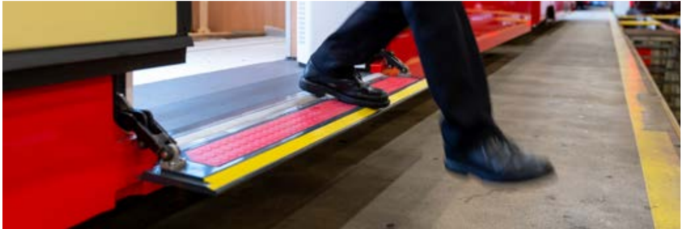
The slip-resistant safety mats on the folding steps act as tactile surface sensors.
