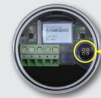
Connection plug for MPI-200-F adapter as an intermediate plug between the ILM-4 electronics and the MPI-200 connection (3) (see figure below).
