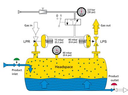
Product transfer is terminated by closing the product outlet valve and setting the servo pressure at the pressure regulator (LPR) and the back pressure regulator (LPS) to zero. This causes the headspace pressure to decrease to the ventilation pressure of 40 mbar (0.6 psi).
