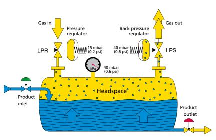
Typical basic settings for tank or reservoir inertising are 15 mbar (0.2 psi) for the pressure regulator (LPR) and 40 mbar (0.6 psi) for the back pressure regulator (LPS). Before a tank is filled with product the empty tank is purged with nitrogen in order to drive out the air. Typically 3 to 5 times the tank volume is used. Once the discharge valve is closed the gas pressure increases to the set value of 15 mbar (0.2 psi).
