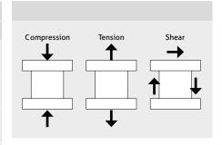
The loads listed above are the maximum ASD loads for the condition listed and are based on the Steel Construction Manual, 14th Edition, of the AISC (American Institute of Steel Construction). Shear and tension values assume mounting hardware is A325 minimum (provided by customer). Higher strength hardware can be used if desired. All load stands must be selected to resist the combined loading effects for the specific jobsite and building code requirements.
