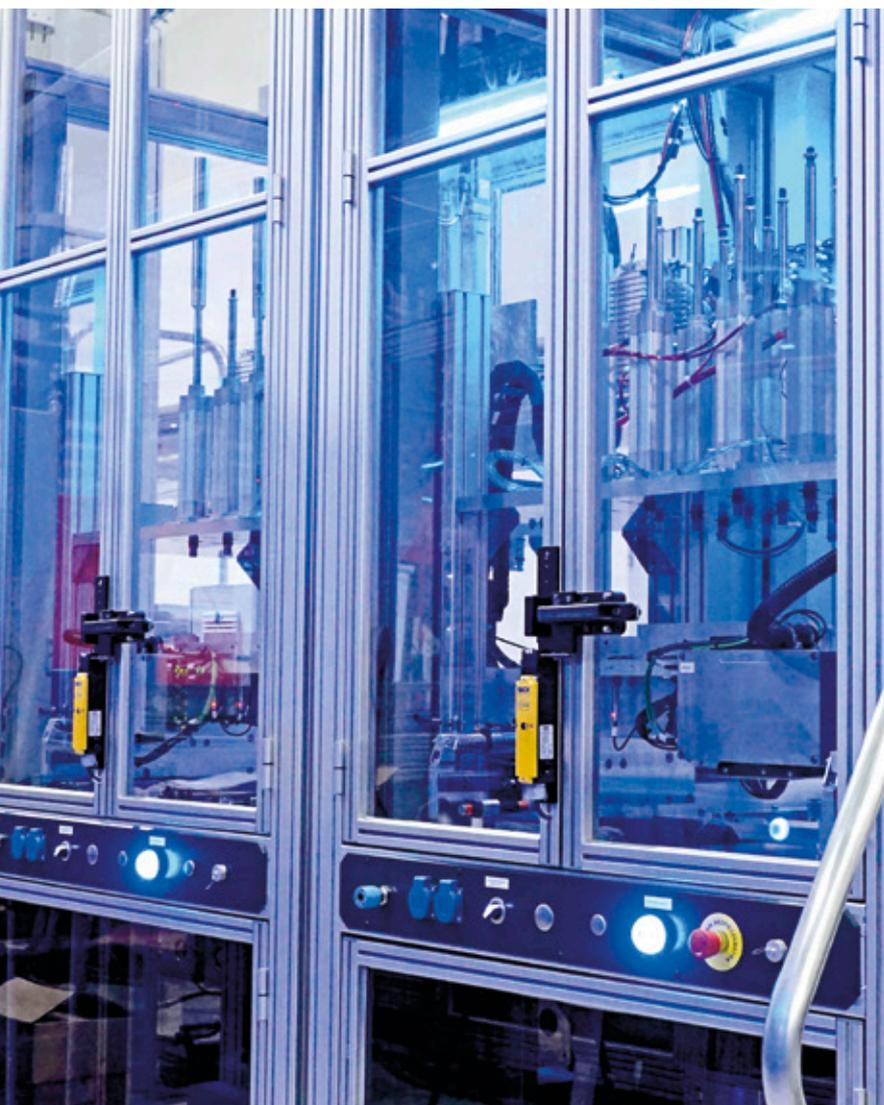
WLS27 LED line lights display the respective status of a module by color
