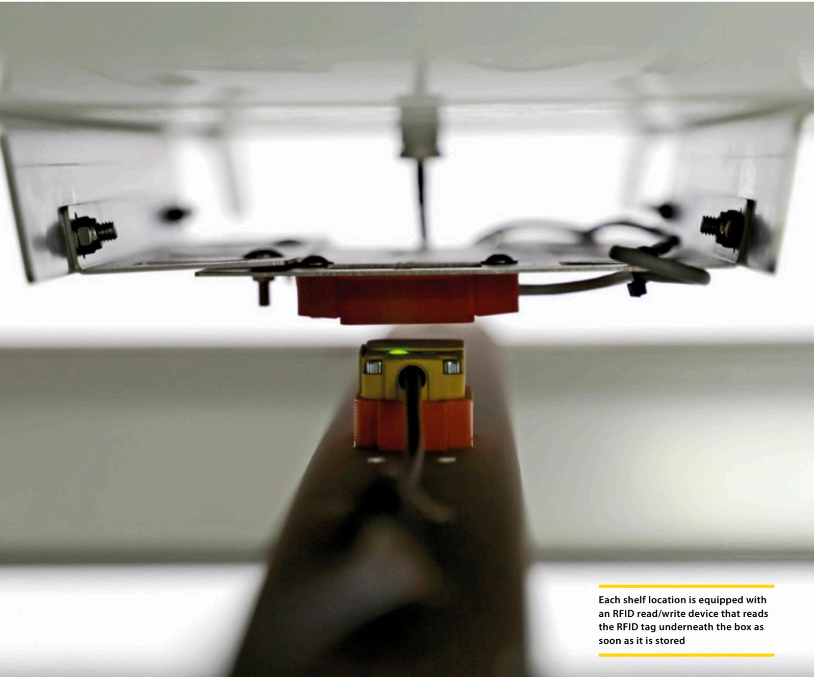
Each shelf location is equipped with an RFID read/write device that reads the RFID tag underneath the box as soon as it is stored
