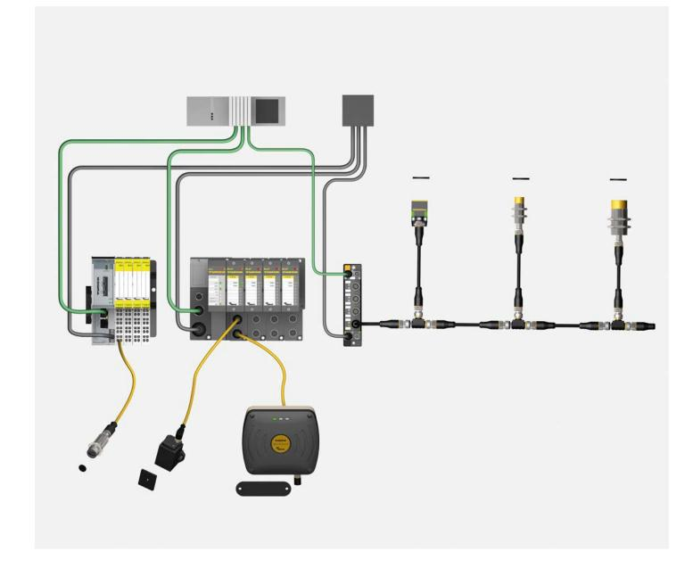
BL ident® is an all-in-one modular RFID system that also plays out its strengths in the food industry. The basic components (cabinet) and the compact fieldbus modules TB...-L... and TB...-S...(field). Both technologies, HF (13.56 MHz, ISO15693) one identification solution.
