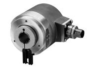
Absolute multiturn encoders detect any angle within a full revolution of 360° and also the number of revolutions. With absolute encoders, each incremental angle is assigned a code pattern. This allows the position to be detected at any time, even after a power failure, without having to initialize a reference run. Absolute encoders detect angles, positions and inclinations precisely – tasks, that are typically found in robotics, positioning and process technology.
