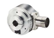
Absolute singleturn encoders detect any angle within a full revolution of 360°. With absolute encoders, each incremental angle is assigned a code pattern. This allows the position to be detected at any time, even after a power failure, without having to initialize a reference run. Absolute encoders detect angles, positions and inclinations precisely – tasks, that are typically found in robotics, positioning and process technology.
